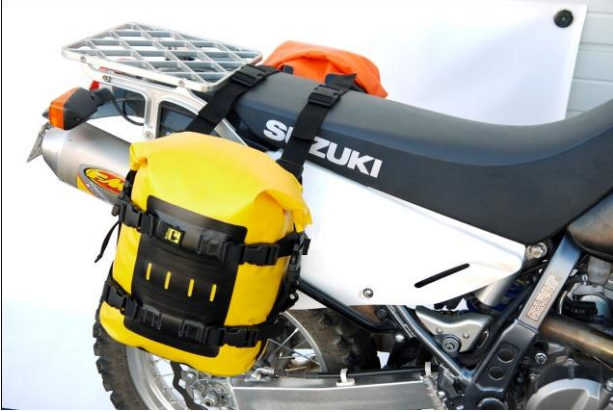
Fig.1 A Properly set of Large Rolie Bags attached to Wolfman/BackRoads Side Racks.
