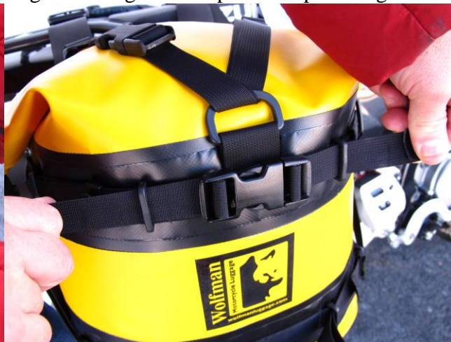
Figure-15 Tighten Straps to compress bag to Rack
