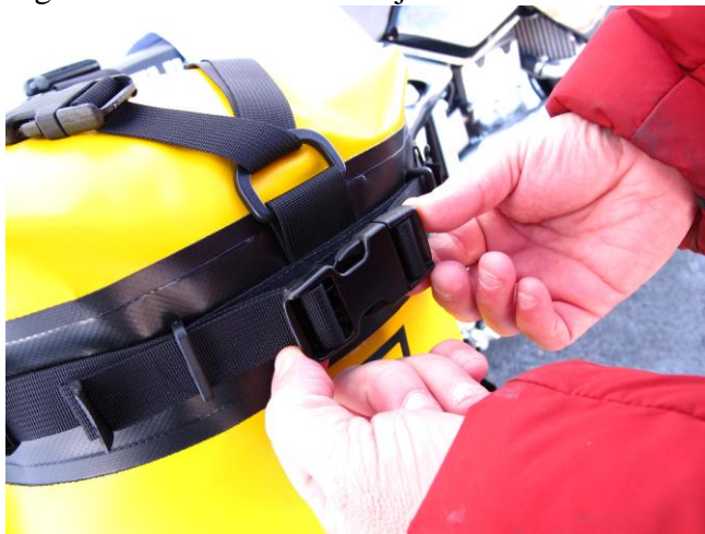
Figure-14 Fasten Center Adjustment Buckle
