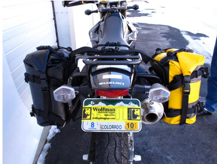
Figure-6 This is a rear view of a properly adjusted set of saddlebags.
